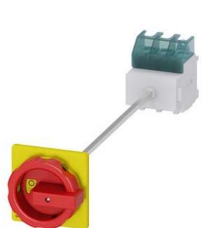
SENTRON, Switch disconnector 3LD, emergency switching-off switch, 3- pole, lu: 63 A, operating power / at AC-23 A 400 V: 22 kW, floor mounting with door coupling, rotary operating mechanism, Red / yellow, 4-hole mounting of the handle
