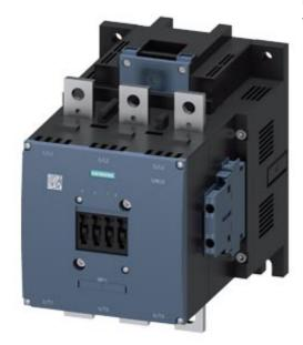
Power contactor, AC-3 500 A, 250 kW / 400 V AC (50-60 Hz) / DC 110-127 V UC Auxiliary contacts 2 NO + 2 NC 3-pole, size S12 Busbar connections Operating mechanism: conventional screw terminals
