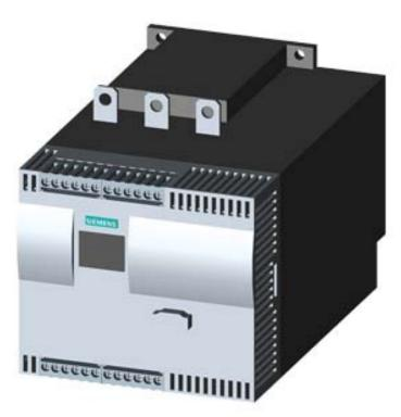
SIRIUS soft starter Values at 400 V, 40 °C Standard: 113 A, 55 kW Inside-delta: 196 A, 110 kW 200-460 V AC, 230 V AC Screw terminals
