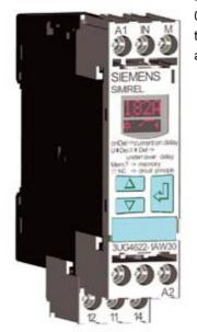
Digital monitoring relay Current monitoring, 22.5 mm from 0.05-10 A AC/DC 0vershoot and undershoot 24 to 240 V AC/DC 50 to 60 Hz DC and AC ON delay and noise pulses delay 0.1 to 20 s Hysteresis 0.01 to 5 A 1 change-over contact with or without fault buffer screw terminal Successor product for 3UG3522-1AL20, 3UG3522-1AG20 and 3UG3522-1AC48-0AA1
