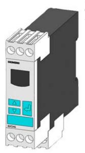
Digital monitoring relay Voltage monitoring, 22.5 mm from 10 to 600 V AC/DC 0vershoot and undershoot 24 to 240 V AC/DC 50 to 60 Hz DC and AC Noise pulses delay 0.1 to 20 s Hysteresis 0.1 to 300 V 1 change-over contact with or without fault buffer screw terminal Successor product for 3UG3532-1AL20, 3UG3532-1AG20
