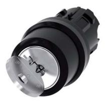
RONIS key-operated switch, 22 mm, round, plastic, lock number SB30, with 2 keys, 2 switch positions O-I, latching, actuating angle 90°, 10:30h/13:30h, key removal O+I, possible special locks: SB31, 421, 455
