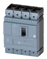
circuit breaker 3VM1 IEC frame 630 breaking capacity class N Icu=36kA @ 415V 4-pole, line protection TM220, ATFM, In=500A overload protection Ir=350A...500A short-circuit protection Ii=10 x In N conductor unprotected nut keeper kit
